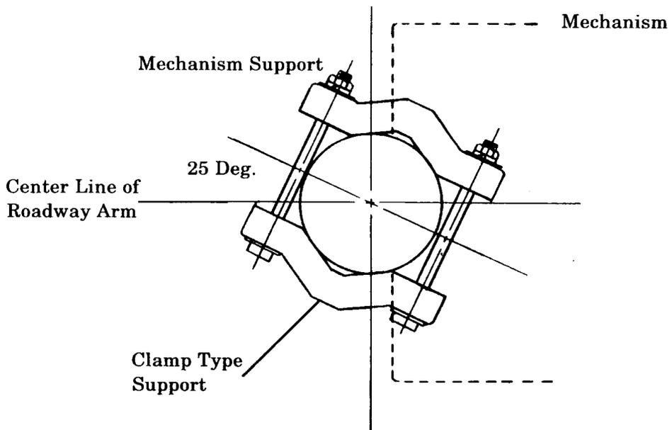
**Clamp Type Mechanism Support Installation
