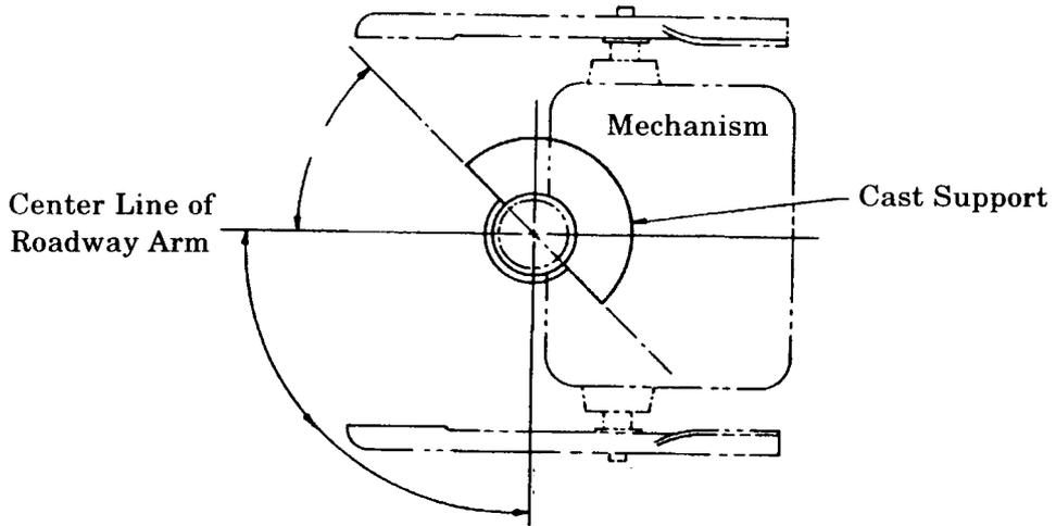
**Cast Mechanism Support Installation
