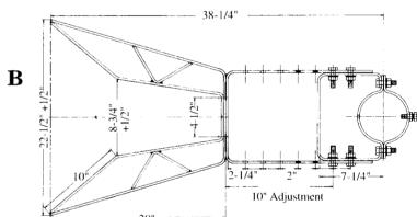
Properly installed, the W-C-H High Wind Gate Arm Support can significantly reduce wind caused knock-downs of breakaway gate arms. Unique features such as the non-binding design of the receiving bracket, the wide receiving angle, and the lock bolt combine to keep the potential for arm blockage to a minimum.
